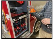
cident. The truck even carries air bags that can be inserted under, say, a piece of heavy equipment, then inflated, lifting it so the trapped victim can be rescued.
